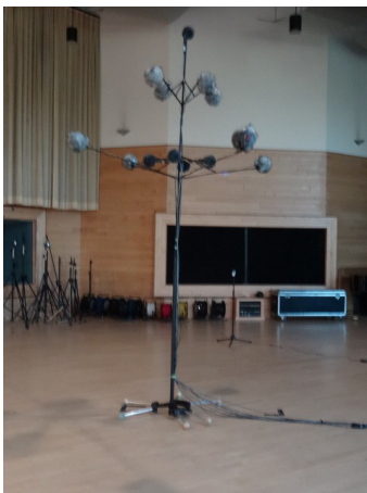
Figure 6 – 8+4+1 Array in Witch's Hat configuration
