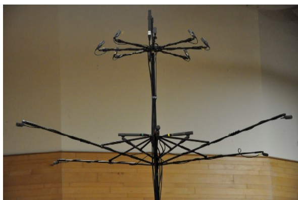
Figure 7 - a Top Hat 8+4+1 3D Microphone Array
